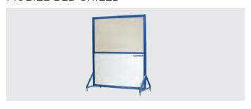
These bed shields are used to protect personnel from radiation during the visit of a patient. The lead shielding has a variable thickness depending on the model. The shields are mounted inside a stainless steel frame on 4 swivel wheels. The window is made of acrylic lead glass and provides a shielding equivalent to a lead thickness of 0.8 mm (for 110 KeV)
