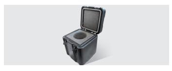
For the transport of radioactive material we provide a special case where materials are placed inside the shielded containers. The case is made of polyethylene (plastic material ensuring resistance and lightness at the same time). It is equipped with an airtight closure with perimeter gaskets, reinforced corners, safety lockups, handle for an easy transporting and an internal pressure compensation valve for airfreight. The interior of the case is coated with a shock-absorbing material.
