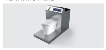
The system allows the collection and the decay of radioactive liquid and organic waste produced in nuclear medicine by the use of Technetium for diagnostic purposes. It consists of a WC equipped with a shredder, which sends the sewage to a collection tank in plastic reinforced by fiberglass. When this tank is full the sewage is deviated to the second tank. A timer is present which evaluates the decaying time of the sewage.
