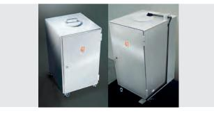
These movable containers are used for radioactive waste. They have been designed specifically to fit the standard blue plastic hospital containers. The containers are made of stainless steel. The plastic hospital container is placed inside the waste container underneath the opening. A shielded lid covers the opening. The door is lockable. The WC-303 waste container has a foot-pedal operated lid.
