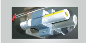
SMART GEIGER is a device for detecting radioactivity inside hot cells. Its main function is to lock the door when the dose rate rises above a pre-set alarm threshold
